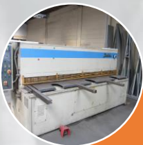
NC Guillotining Up to 6mm thick x 3100mm long
